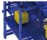
◆The drawer can be entirely pulled out to facilitate the lifting and loading of bulky moulds.
