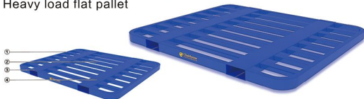
①Frame ②Cross brace ③Strengthened bending plate ④Forklift hole
