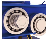
◆The bearings under the drawer make it smooth and labor-saving when drawing out and in.
